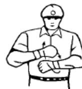
FOR MOBILE CRANES TRAVEL BOTH CRAWLER BELTS IN DIRECTION INDICATED BY REVOLVING FISTS
