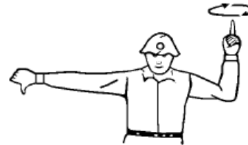
FOR MOBILE CRANES HOIST THE LOAD AND LOWER THE BOOM
