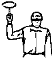
HOIST THE LOAD
