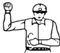
FOR MOBILE CRANES LOCK THE CRAWLER BELT ON SIDE INDICATED BY RAISED FIST TRAVEL OTHER CRAWLER BELT IN DIRECTION INDICATED BY REVOLVING FIST
