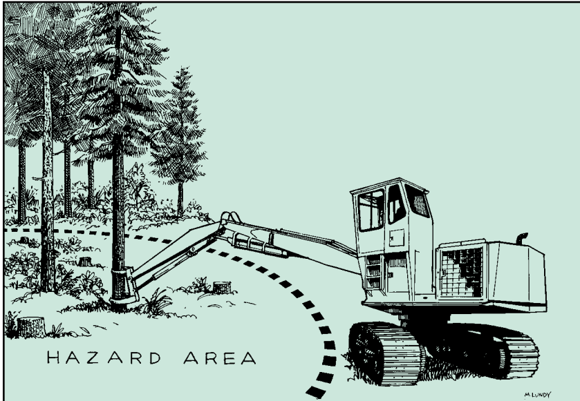
Fig. 11. — Felling trees from outside the hazard area.
