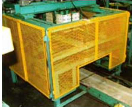
Example of enclosing hazard from power transmission machinery
