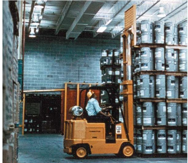
Internal combustion engine forklifts can cause carbon monoxide poisoning when used indoors if the engine is not kept tuned and the area well ventilated.
