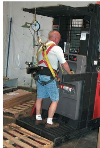
The operator of an order-picker-type forklift must wear a safety harness to protect against the fall hazard at an elevated location.
