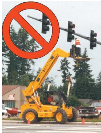
Never stand on the forks or a pallet to work at an elevated level.
