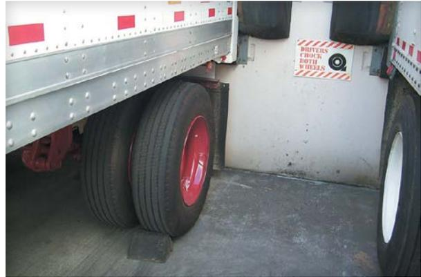
Trucks or trailers must be chocked or blocked at the wheels, or with a mechanical device that secures the truck or trailer to the loading dock. Notice the sign tells drivers to chock the wheels.
