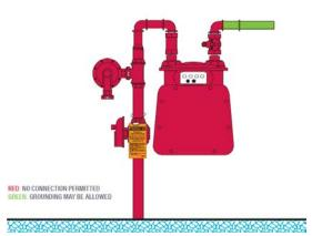
Each gas utility meter has insulated fittings to keep their system isolated from the mechanical and electrical systems of a customer. If an electrician bonds the wrong side of the meter, they have not bonded the building metal piping system, and circumvented the cathodic protection system, which can lead to a gas leak, injury or a structure fire.
