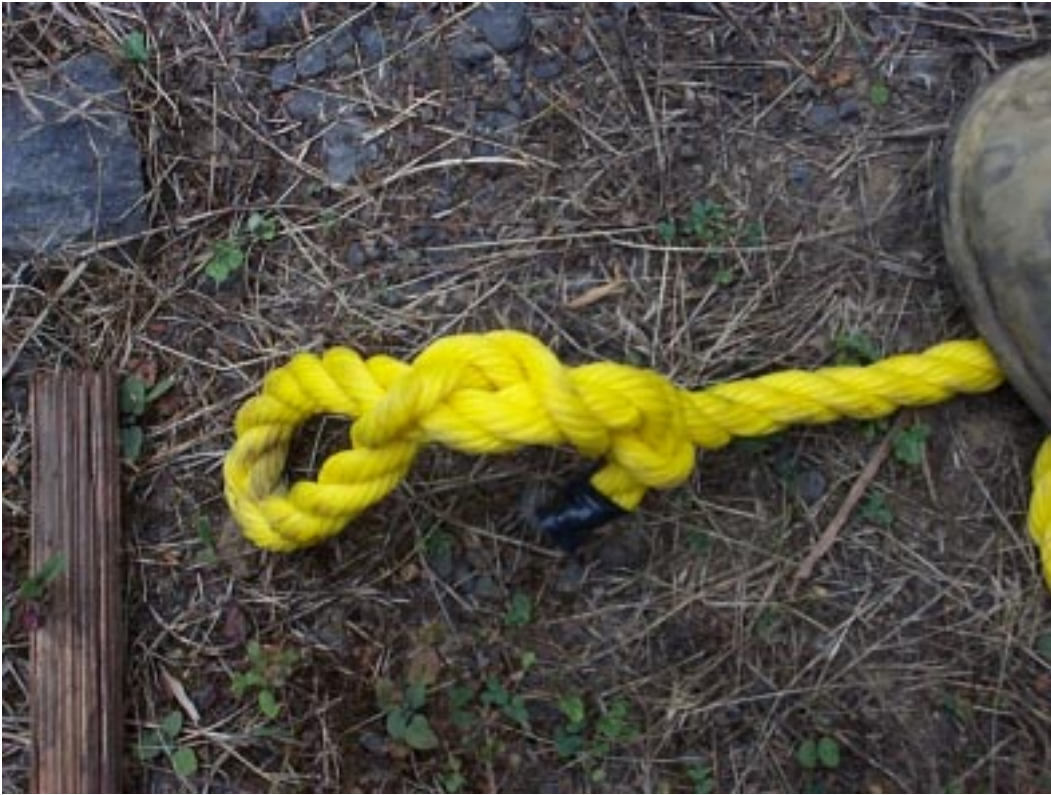
Figure 3a Example of a compression splice. This is not an appropriate splice for this application.
