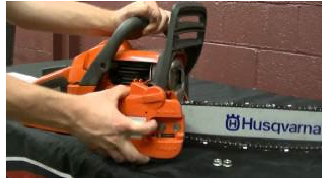
Image: Russo Power Equipment YouTube "How to remove a chainsaw clutch cover and reset the chain brake" https://www.russopower.com/
