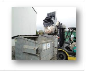
A forklift attachment lifts heavy garbage into the dumpster.
