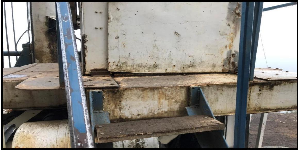
The deck surface of the yarder is worn down to bare metal and is needing repaired.
