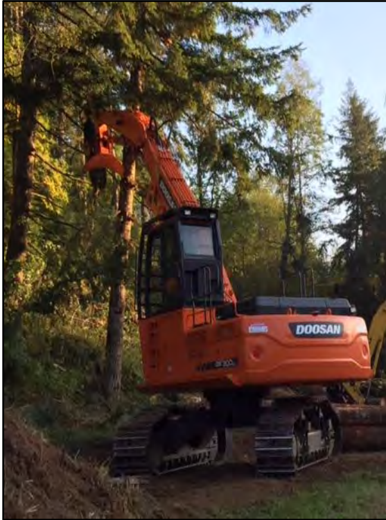
*Machine removes limbs before cutting
