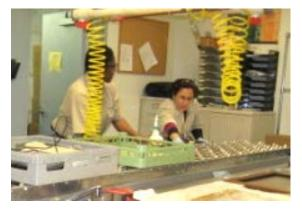
The cleaning stations were deep. This made workers reach a long way to pick items from racks while on either side of the conveyor. For short workers they also had to bend forward at the waist to reach items.
