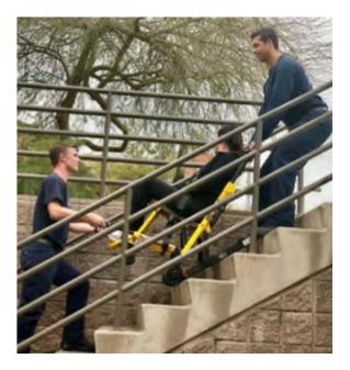
The gliding movement significantly reduces back compression force, with lower perceived exertion ratings, compared to traditional chairs. EMTs in one study felt that the leader facing forward position was more efficient.
