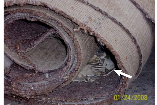
VAT debris rolled up in carpeting
