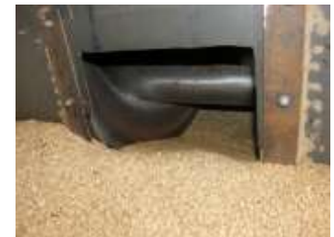
2. Bad idea. You can slip and slide right into the exposed shear points on this floor auger.
