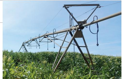
Field irrigation systems, as shown in this photo, are large metal structures that can span 1,200 ft and are often powered with 480 volts.
