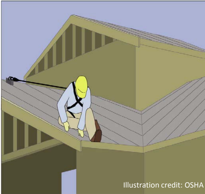
Illustration 1: Roofer using fall protection system
