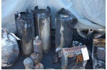
Photo 3: Incident propane cylinders and space heater.
