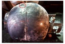
Photo 4: Incident 20-Ib. propane cylinder as found inside the stand. A cylinder breech crack was caused by the fire (circled).
