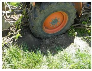
Photo 2: Right rear tire that continued turning after tractor ran over and became stuck on tree
