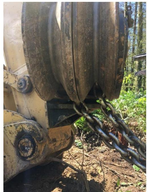
**Lower sheaves of base machine showing wear on the housing from socket striking.**
