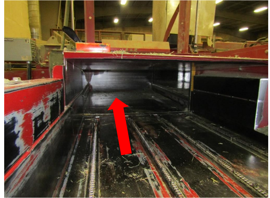
The arrow indicates the victim's location on the scale when his weight activated the guillotine.
