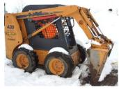
Skid steer loader at the incident scene showing the position of the arms and bucket before the victim was pinned between the arms and frame.
