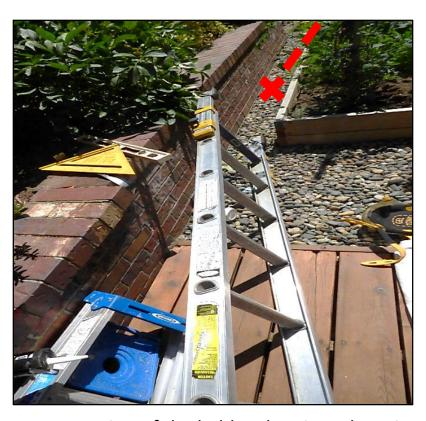
**Photo 1**. Base section of the ladder showing where it was set up behind a wood-framed garden bed (shown by "X") and leaned against a house chimney chase at a 65- degree angle.
