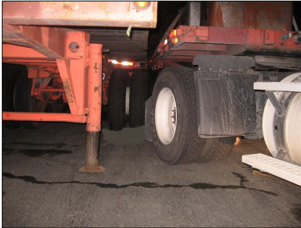
Photo 3. Close-up view of the pinch point between the two trailers where the driver was crushed while cranking up the trailer's landing gear.
