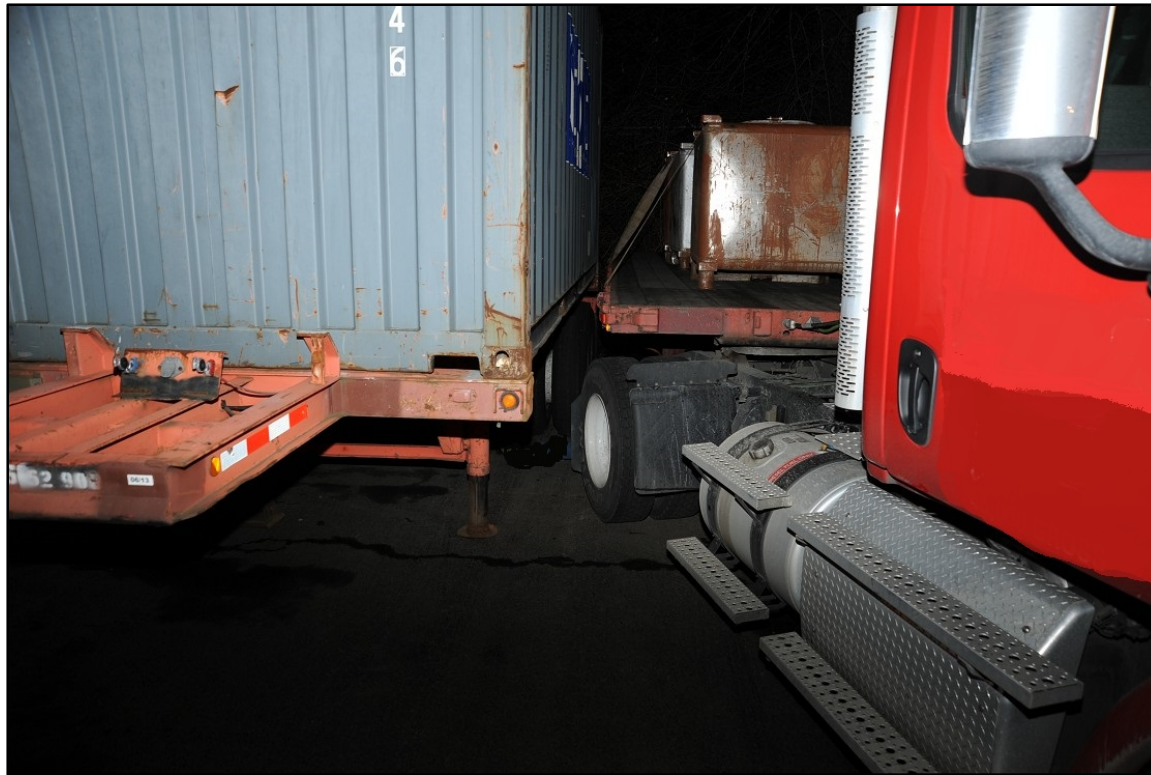
Photo 2. The pinch point where the driver was crushed between the two trailers.
