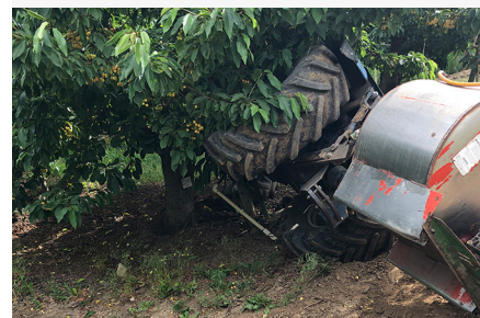
Incident 2: Overturned tractor after it rolled downhill and struck a tree.
