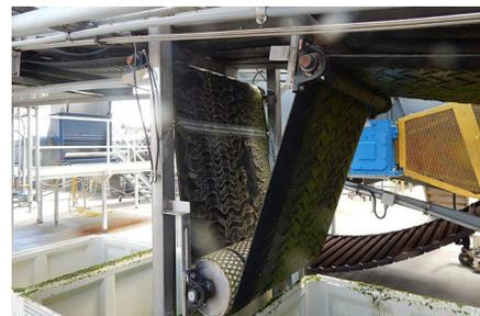
**Incident 1:** The maintenance worker's arm became entangled in the upper right roller.
