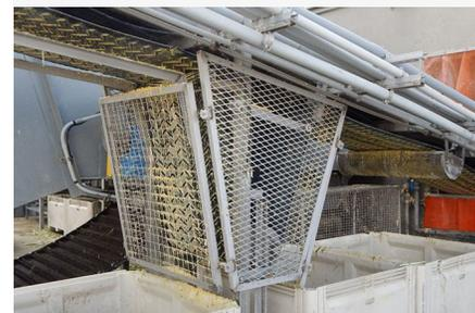
**Incident 1:** Conveyor belt and rollers that the employer guarded after the incident. The guards are welded to the frame.
