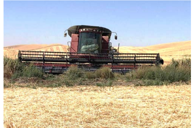
Combine that backed up and ran over the operator after he “hot-wired” its starter and then fell off the rear access ladder landing on the ground and was struck by the header.
