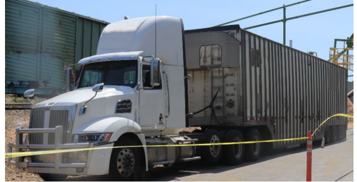
Woodchip truck that rolled away and crushed driver. The driver parked the truck on a paved road under a tarping station. The road had a 2% downgrade. The driver left the truck running and did not set the parking brake before exiting the cab to access the top of the trailer.
