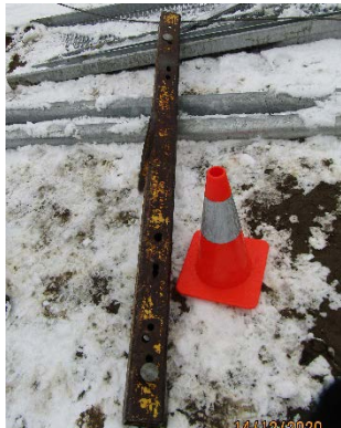
Gin pole jump plate used in the operation.
