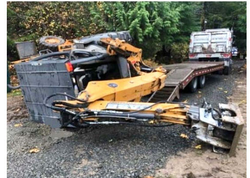
Overturned backhoe and the trailer onto which the driver was attempting to load the backhoe when it rolled over, crushing him.
