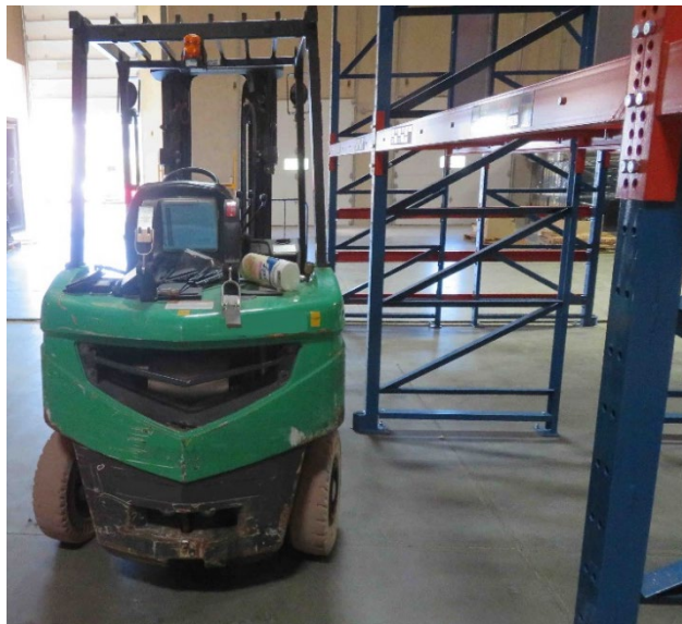
Rear side of forklift that struck and crushed the operator against one of the metal uprights.
