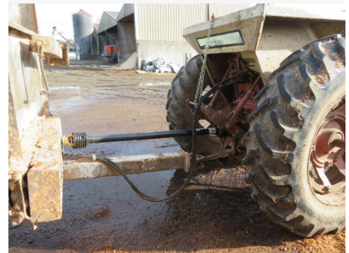
The foreman was standing on the front of the trailer above the unguarded power takeoff (PTO) shaft when the incident occurred. (Photo shows PTO shaft with guard installed)
