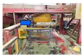
Hay press bale elevator with output platform and pusher in foreground. Arrow shows elevator and yellow table that came off it when the worker was crushed. Warning signs are on the machine frame above the elevator. The worker entered the area from the back.
