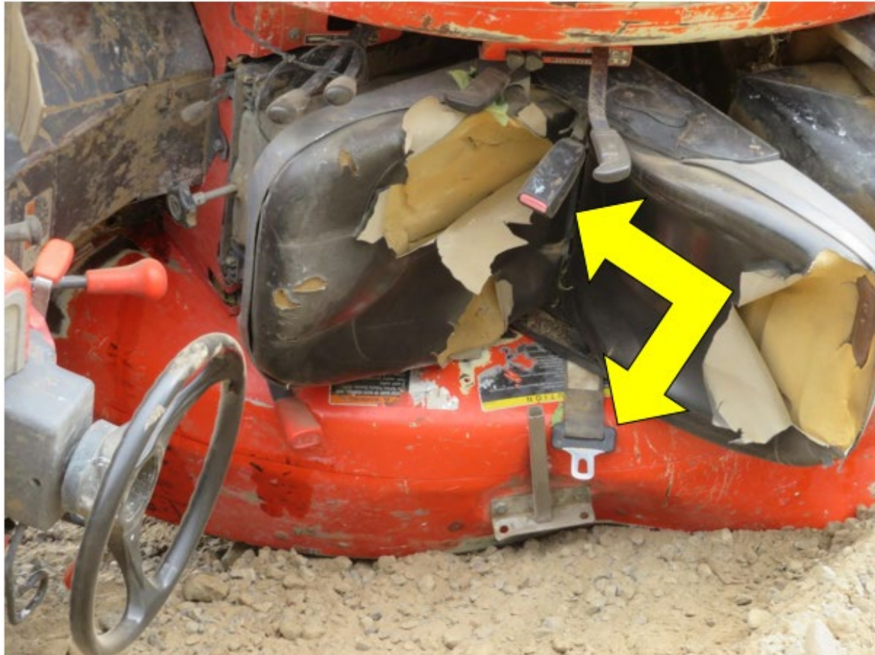
Photo 3. Unbuckled operator's seat belt on tractor that rolled over. Note worn out warning labels on left fender wall.
