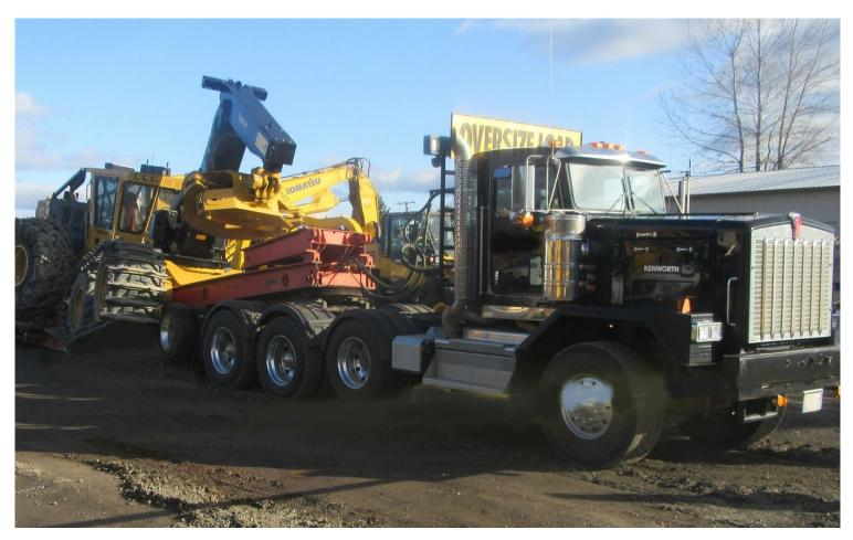
Photo 1. Semi-truck with skidder on detachable lowboy flatbed trailer in rear.
