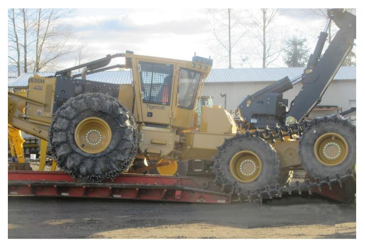
**Photo 3.** Skidder with tracked bogie wheels between lowboy trailer's lowered flatbed deck and detached gooseneck.
