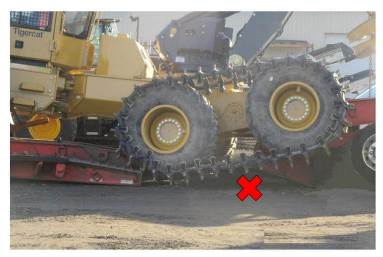
Photo 2. The owner was crushed under the skidder's tracked bogie wheels (X).
