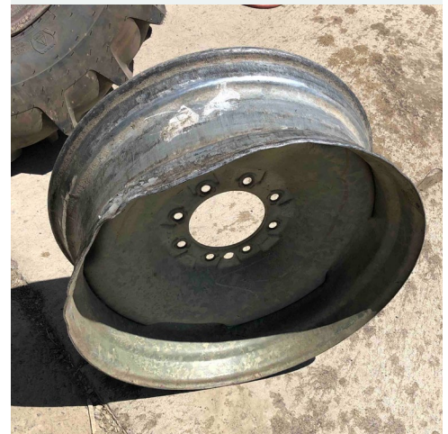
The wheel that shot out of the tire, striking the tire technician.
