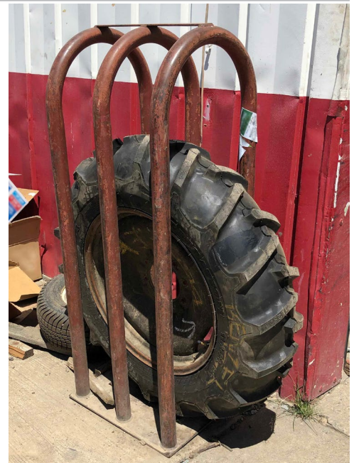
Employer's inflation safety cage, with a tire similar to the one in the incident.
