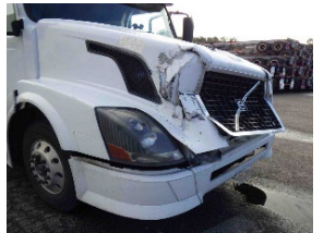
Damage on rollaway truck from hitting chassis.
