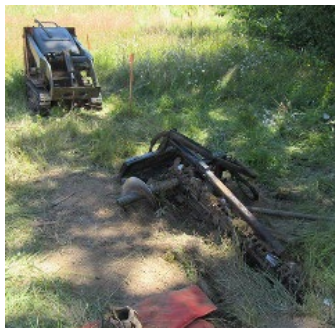
Mini skid steer with trencher attachment.
