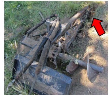
Trencher attachment. Arrow shows chain and digging teeth.
