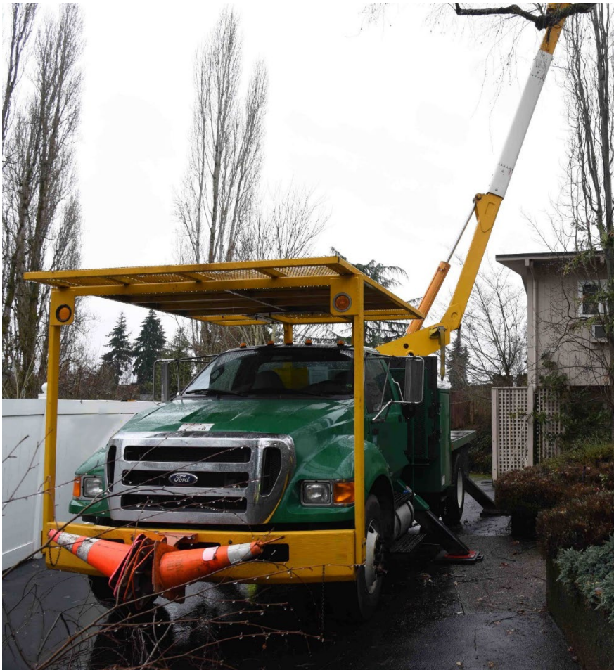
Photos 4 and 5. Left photo shows bucket truck with boom extended. Right photo shows truck's boom lift platform with extended outriggers and rear wheels chocked.
