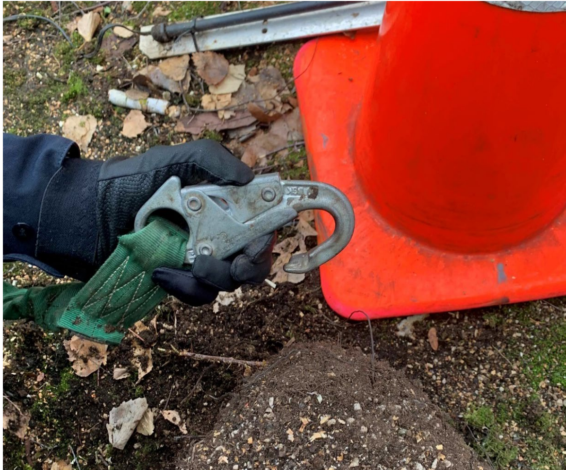
Photo 3. Unsecured snap hook on trimmer's fall arrest harness lanyard.
