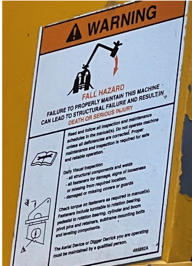
Photos 6 and 7. Left photo shows fall hazard warning label on base of boom lift. Right photo shows other warning and danger labels on base of boom lift. Arrow shows emergency stop switch.
