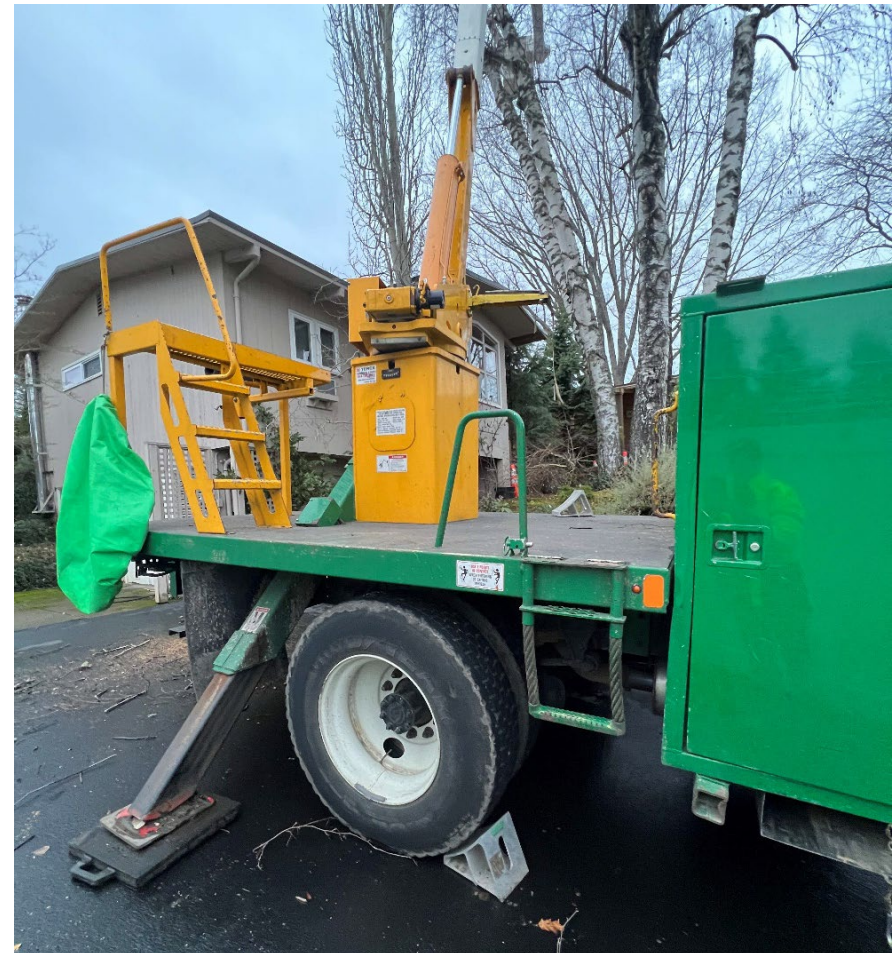
Photos 4 and 5. Left photo shows bucket truck with boom extended. Right photo shows truck's boom lift platform with extended outriggers and rear wheels chocked.
