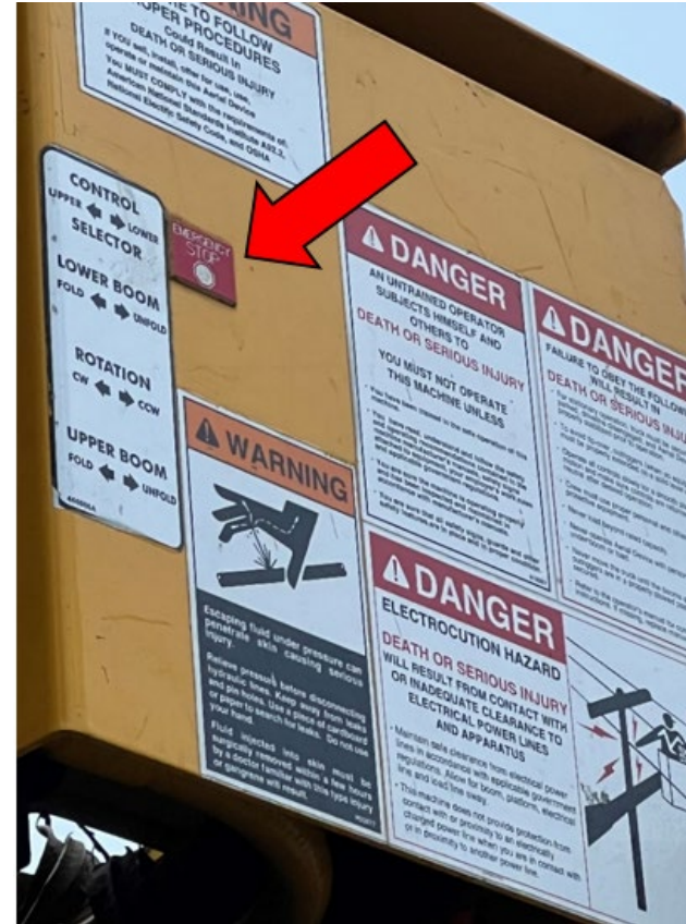
Photos 6 and 7. Left photo shows fall hazard warning label on base of boom lift. Right photo shows other warning and danger labels on base of boom lift. Arrow shows emergency stop switch.
