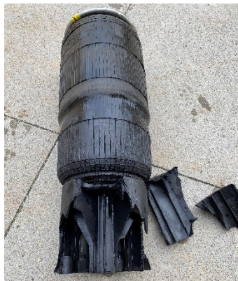
Air spring that struck mechanic.
