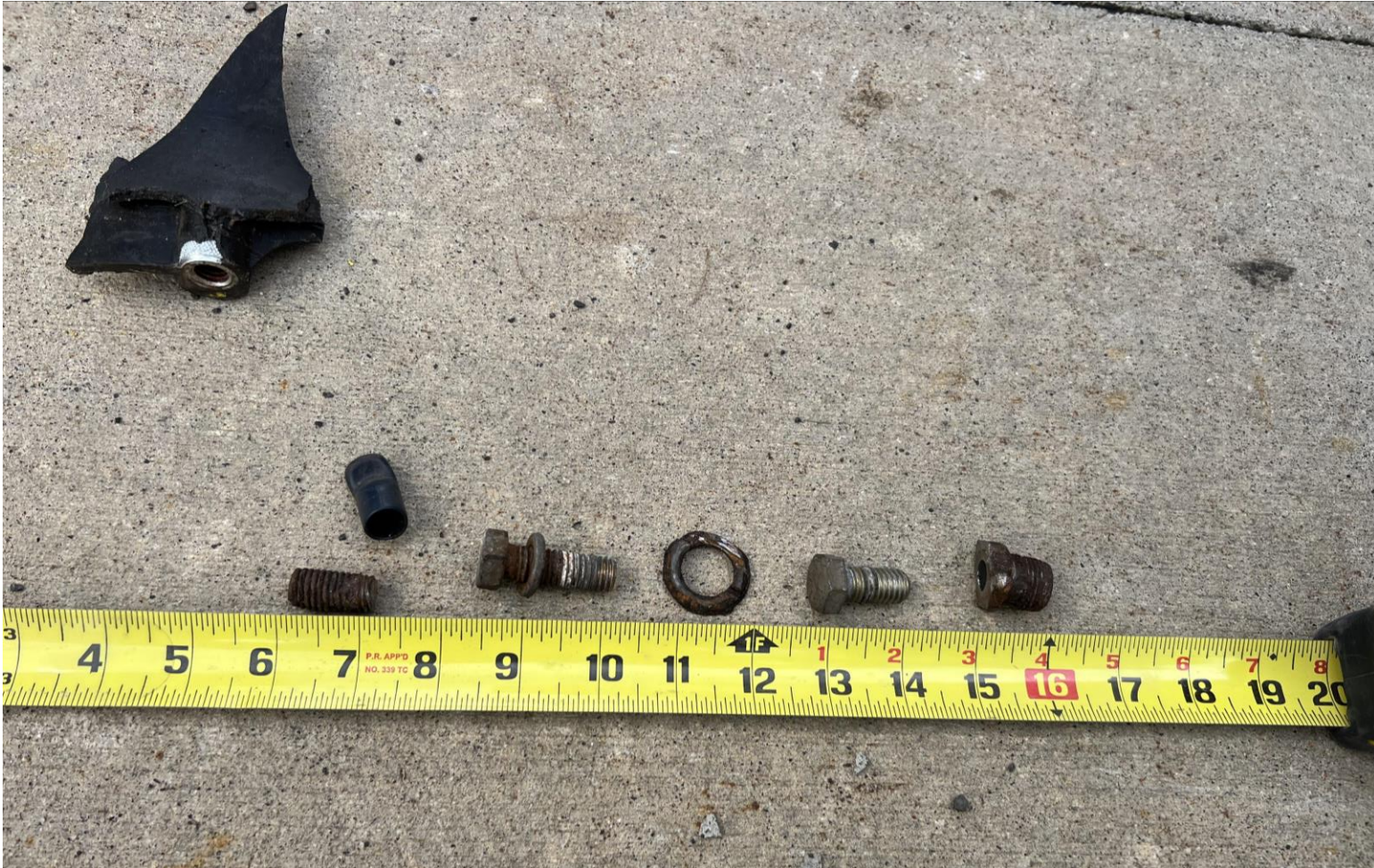
Photo 4. Worn, broken, and sheared air spring mounting bolts found at incident scene.
