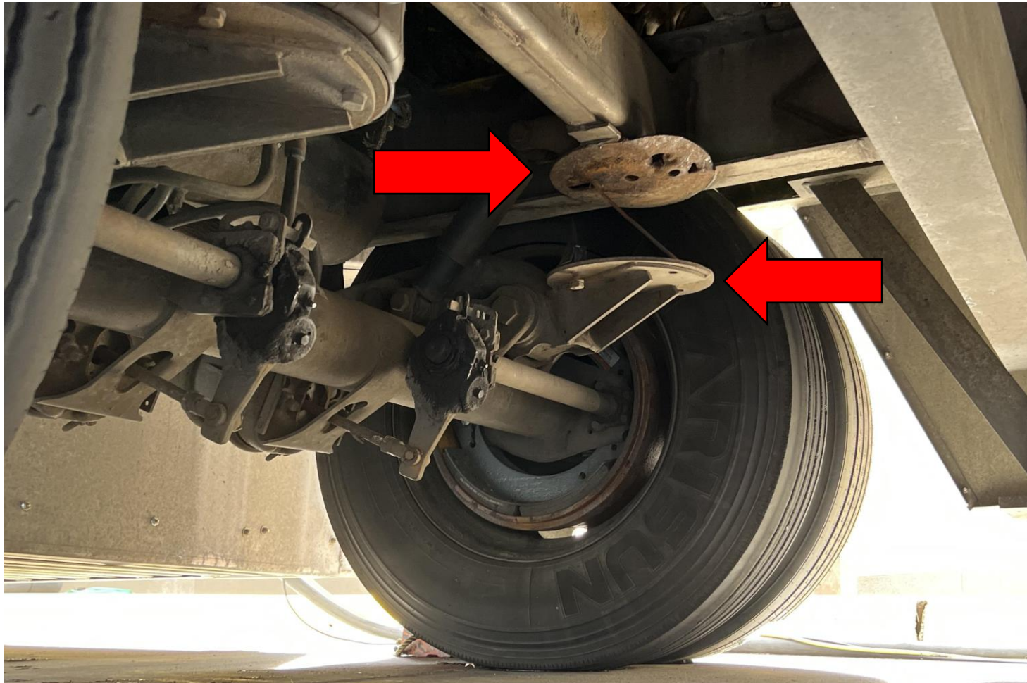
Photo 3. Upper and lower mounting plates where air spring was partly wedged and then ejected during inflation.
