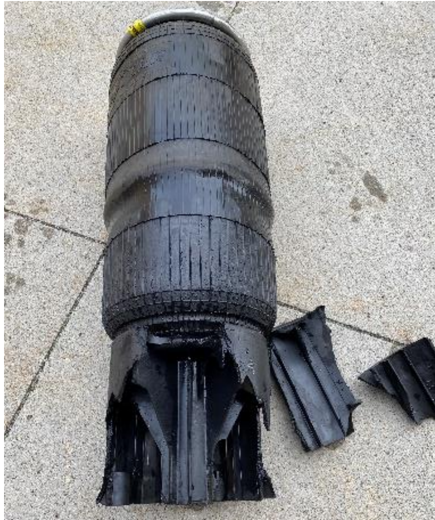
Photo 2. Air spring that struck mechanic.
