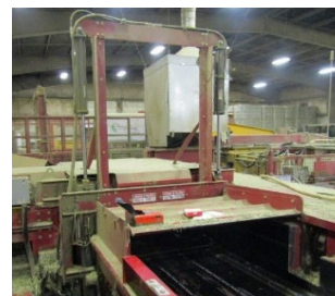
Hay intake area where worker entered and was struck by the guillotine.
