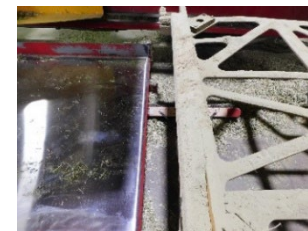
Pinch point between lowered bale elevator on right and output platform on left.
