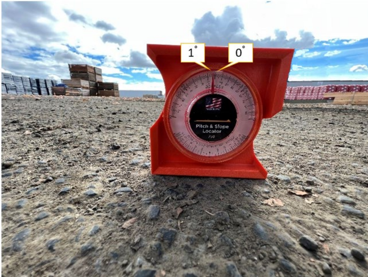
Photo 3. Pitch and slope indicator showing one-percent grade at incident site.
