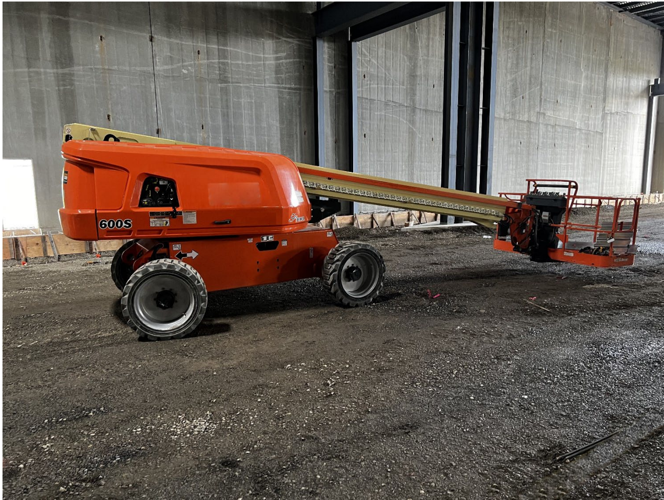
Photo 5. Boom lift with basket used a fall catch platform.
