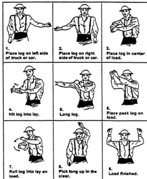
Figure 42: Standard Signals for Loading Logs
