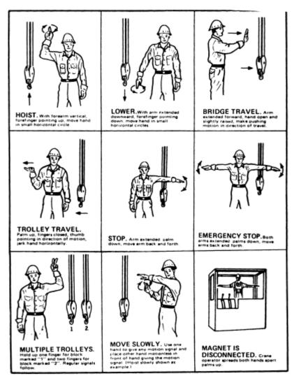
(3) The following hand signals must be used for derricks and a copy must be posted at the operator's station.
