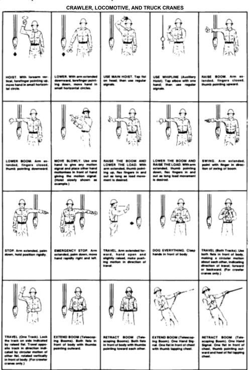
(2) The following hand signals must be used for overhead and gantry cranes and a copy must be posted in the cab at the operator's station.
