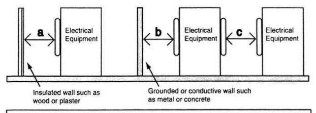
Distances are measured from live parts if they are exposed or from the enclosure front if live parts are enclosed.
