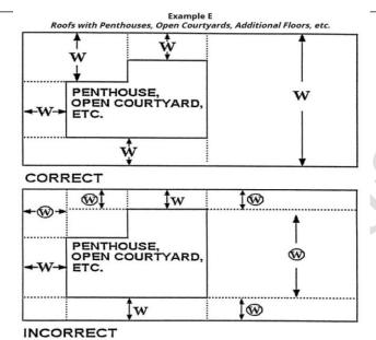
Such roofs are to be divided into subareas by using dividing lines of minimum length to minimize the size and number of the areas which are potentially less than or equal to fifty feet (15.25 m) in width in order to limit the size of roof areas where the safety monitoring system alone can be used. Dotted lines are used in the examples to show the location of dividing lines.
