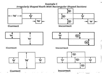
Such roofs are to be divided into subareas by using dividing lines of minimum length to minimize the size and number of the areas which are potentially less than or equal to fifty feet (15.25 m) in width, in order to limit the size of roof areas where the safety monitoring system alone can be used (WAC 296-880-40045(1)). Dotted lines are used in the examples to show the location of dividing lines.
