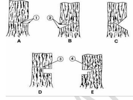
2 (A) Conventional under cut. Can be made with parallel saw cut and
