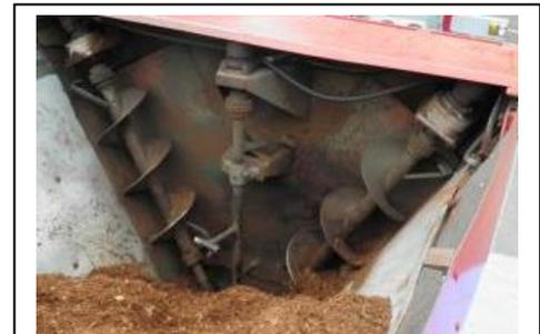
**Danger zone! Do not enter the hopper or use hands or any part of your body to clear jams or move materials.** Even slow-moving mechanical parts like the rotating shaft and augers shown here, have killed or maimed workers that entered hoppers.
